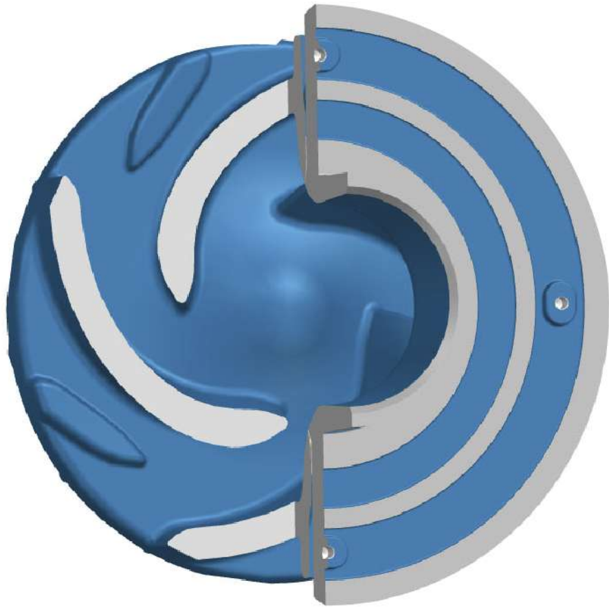
Figure 4: "WRT" Design of Impeller and Throatbush Combination
